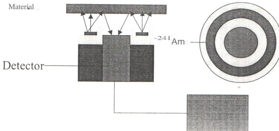
Figure 2. A Typical Backscatter Mode Gamma-ray Thickness Gauge
