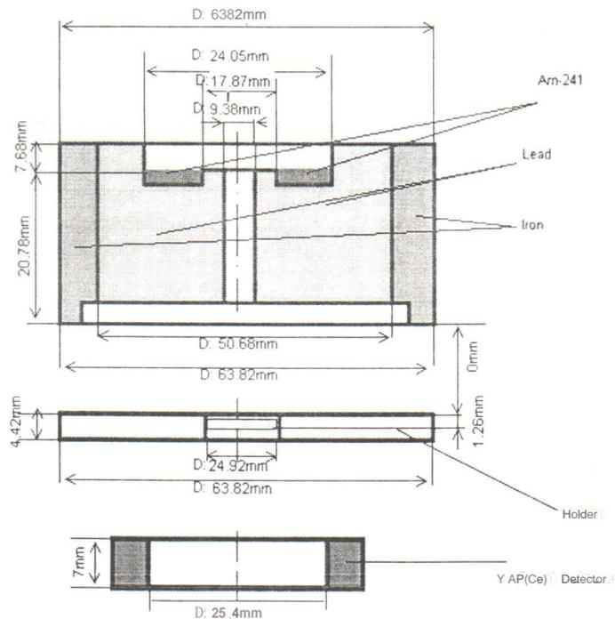
Figure 3. Detailed Arrangement of the <sup>241</sup>Am Annular Source, Source Holder/Shield, Combined with YAP(Ce) Crystal (Net Size of About 25 mm Diameter x 1 mm Thickness).
