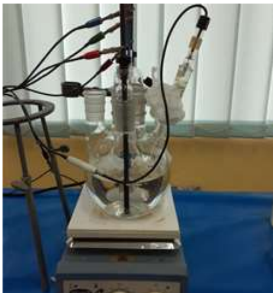
Figure 2. Cell circuit for corrosion rate measurement
