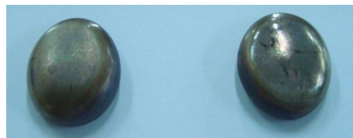
Gambar 1. Ingot paduan U-7Mo-1Zr hasil peleburan
