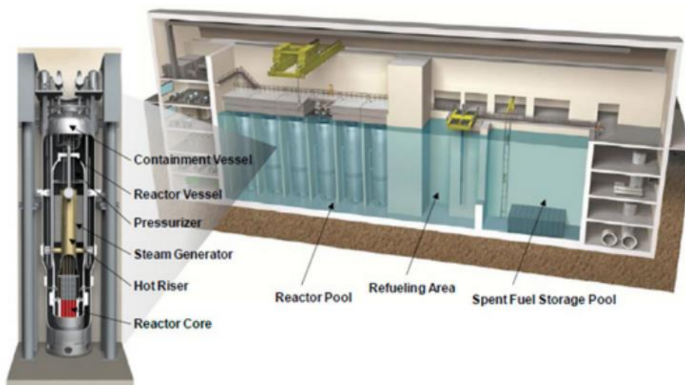
Figure 1. NuScale reactor design [6].
