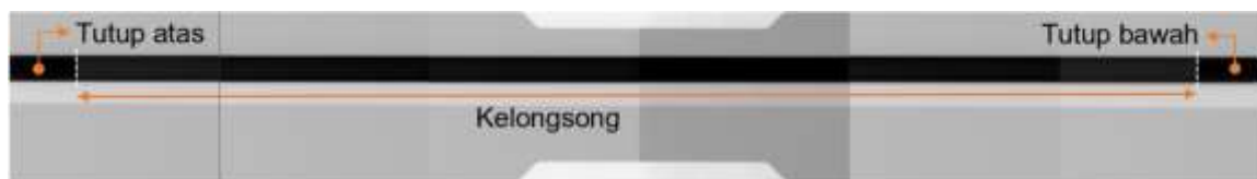
Gambar 6. Penampakan citra radiograf utuh short pin PWR fuel dummy pasca iradiasi
