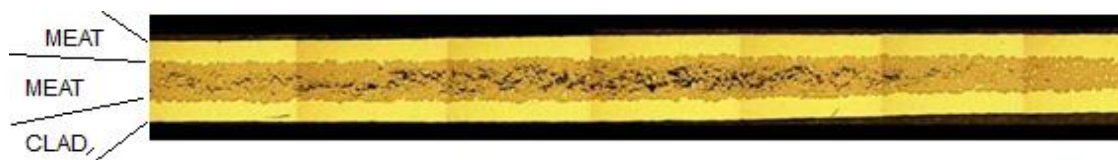
Figure 2. Metallograph of irradiated fuel plate at mid length and across its width and thickness [3] .
