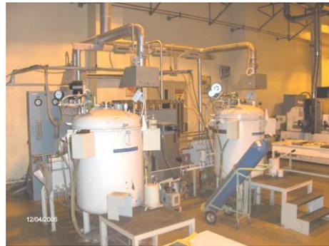
Gambar 1. Peralatan *Sintering furnace*-ME 06 (ruang HR-05)
