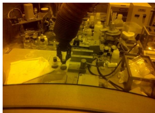
Gambar 2. Proses Pelarutan PEB \text{U}_3\text{Si}_2\text{-Al} pasca iradiasi
