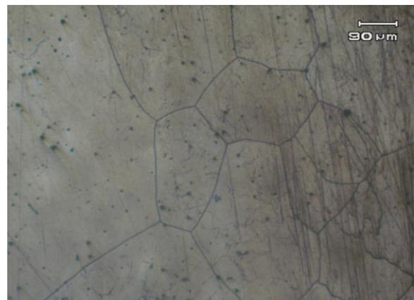
Fig. 3. Optical micrograph of normalized non standard austenitic sample after homogenization at 1200 °C for 20 h.
