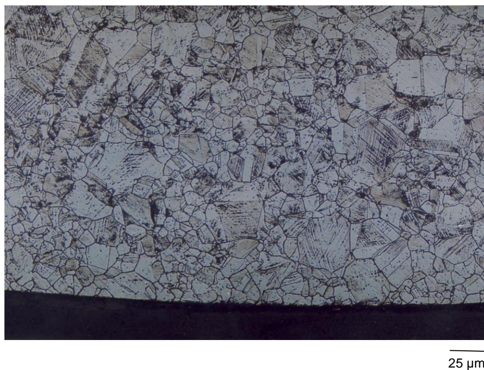
Gambar 8. SS 304 Nitrocarburizing 650°C
