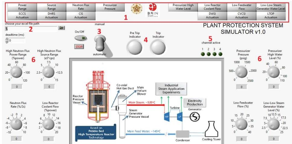
Fig. 6. Initial condition of RPS
