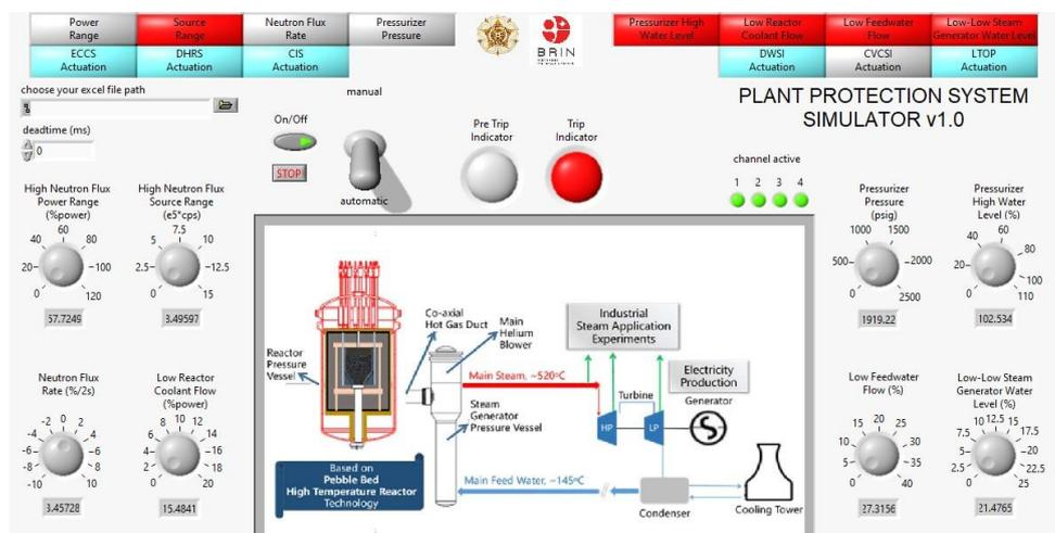
Fig. 7. Trip condition of RPS
