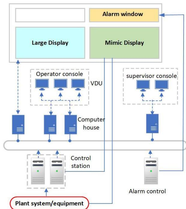
**Fig. 1.** HMI design of SMR main control room [13]
