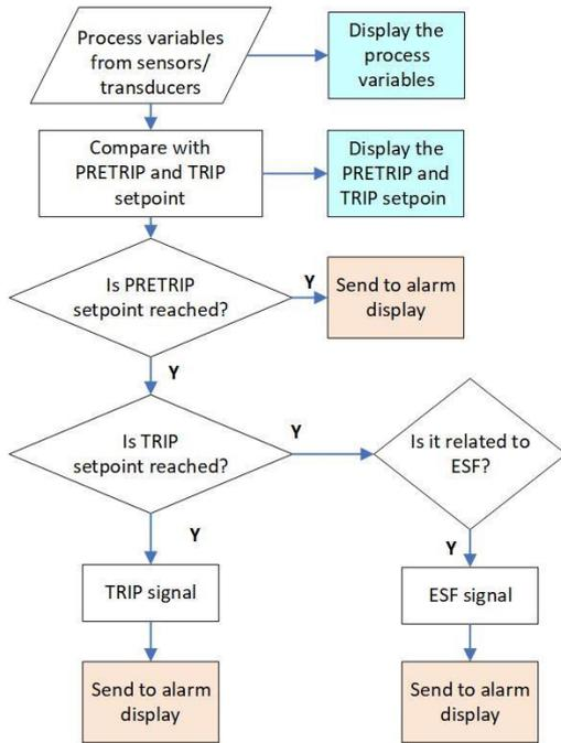
Fig. 5. Information flow of HMI of the PPS
