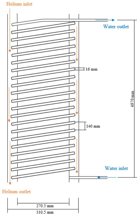
Fig. 3. Schematic of helical pipe steam generator
