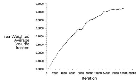
**Fig. 6.** Vapor fraction graph to simulation iteration
