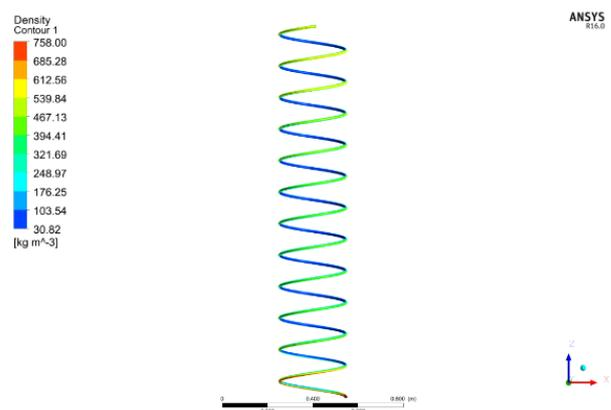
**Fig. 9.** Two-phase density distribution
