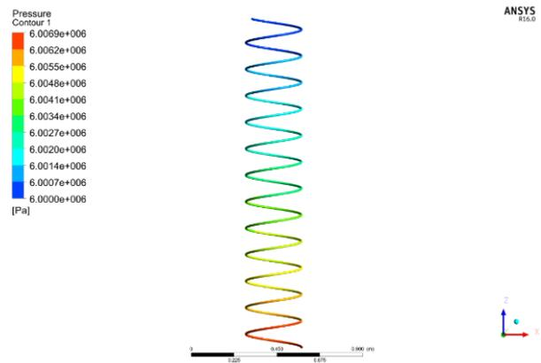
**Fig. 8.** Single-phase liquid pressure distribution
