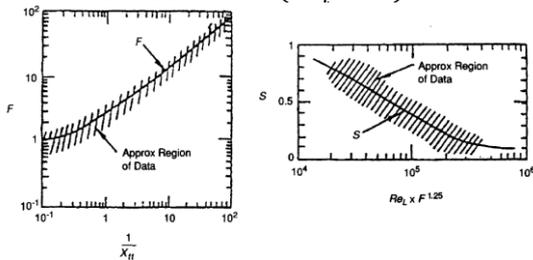
Fig. 1. Chen graphic correlation for convection factor  $F$  and suppression factor  $S$  (Chen et al. 1966)
