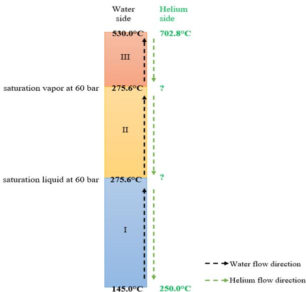
Fig. 4. Three sections of the heat transfer for the empirical calculation the steam generator design
