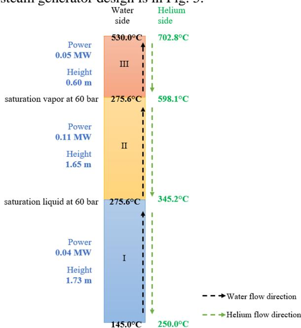
**Fig. 5.** Schematic of empirical calculation results in each heat transfer section
