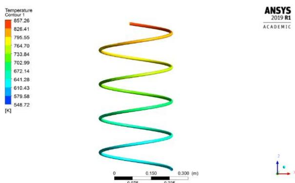
Fig. 11. Single-phase vapor temperature distribution
