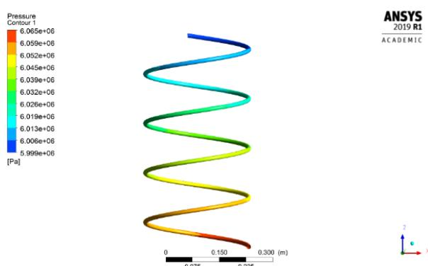
Fig. 12. Single-phase vapor pressure distribution
