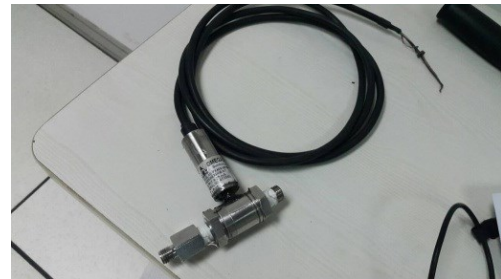
Gambar 7. Differential Pressure Transmitter untai FASSIP-01
