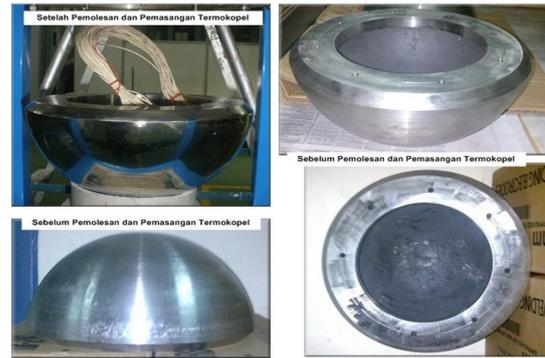
Gambar 1. Bejana uji geometri semi sphere
