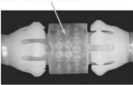
Gambar 7. *Probe array eddy current*<sup>(3,6)</sup>
