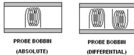
Gambar 8. *Probe bobbin absolute* dan *probe bobbin differential*<sup>(3)</sup>
