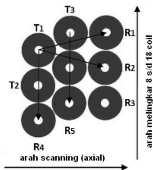
Gambar 11. Prinsip kerja *probe array eddy current*<sup>(7,9)</sup>
