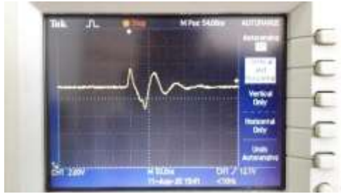
b. Catu-daya linier: Transient beban-OFF.
