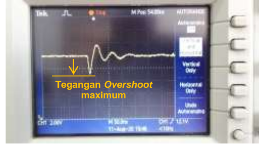
c. Catu-daya SMPS: Transient beban-ON.
