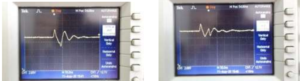
b. Catu-daya linier: Transient beban-OFF.
