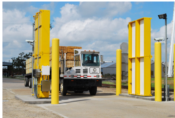
Gambar 1. Contoh Portal Monitor Radiasi (PMR) komersil[1]
