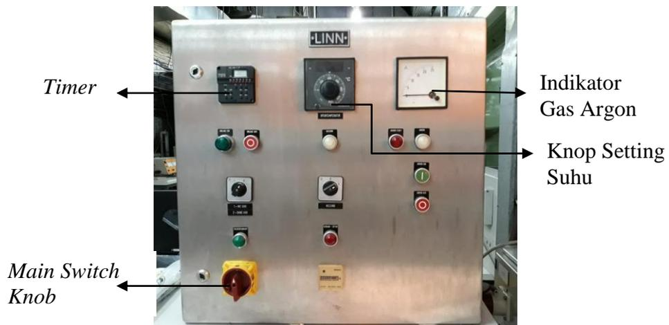
Gambar 3. Kontrol Panel alat TGA
