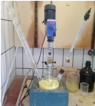
Gambar 2. Proses pelindian HCl
