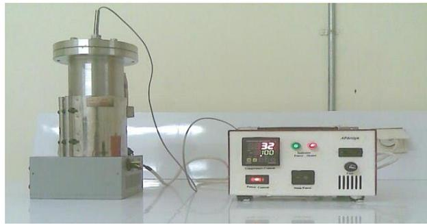
Gambar 1. Rangkaian alat uji korosi (*Autoclave* mini)
