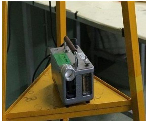
Gambar 2. Air Sampler Staplex
