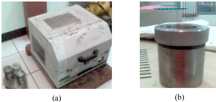
Figure 1. (a) High energy milling (HEM); (b) HEM vial
