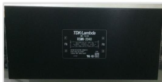
Gambar 3. *Passive EMI filter 220VAC/40A*
