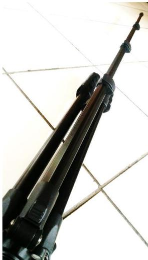
Gambar 10. Komponen tripod model excell UFO 360 (height range 40-160 cm)
