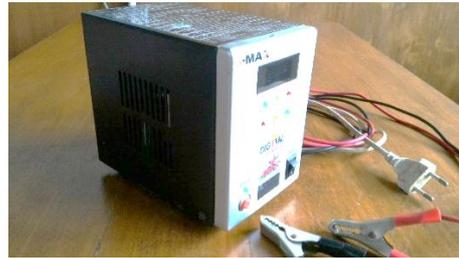
Gambar 12. Komponen *digital intelegent charger* model i-MAX 901-DC-A110-R1 CHG8B HEX
