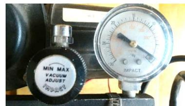
Gambar 4. Komponen *valve regulator/flowrate control* (*integrated with motor system*) dan barometer (capacity range 0-760 mmHg)
