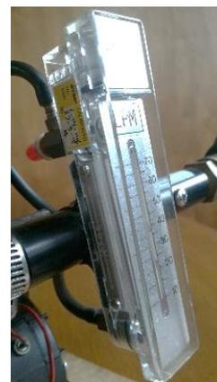
Gambar 5. Komponen *flowratemeter* model HI-Q (capacity range 0-70 LPM)
