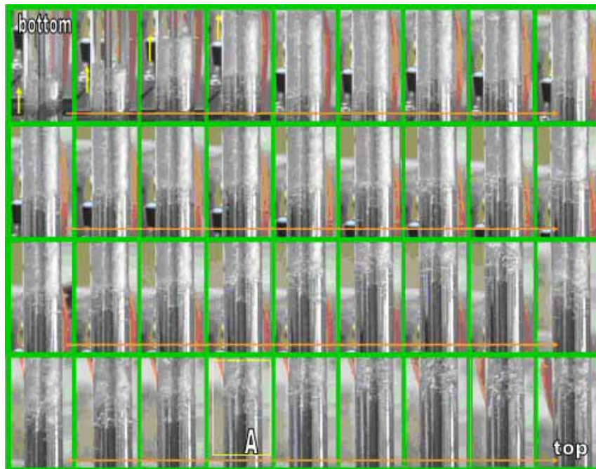
Figure 5. Photos for Boiling Visualization at T_{\text{initial}} = 850^{\circ}\text{C} and G = 0.140 \text{ kg/s}
