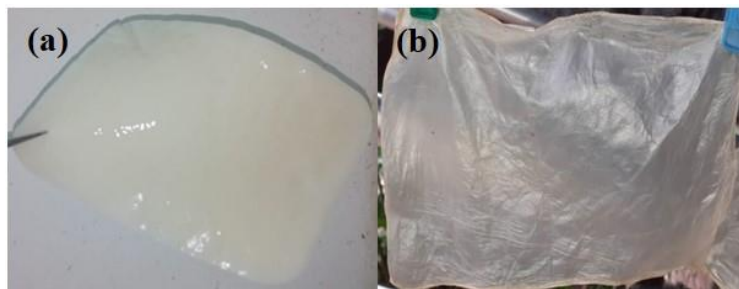
Figure 1. The Nata de Cassava by A. xylinum from the liquid tapioca waste (a) before and (b) after drying
