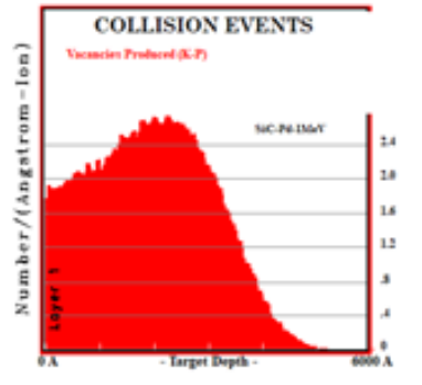
(f) Damage/collision events
