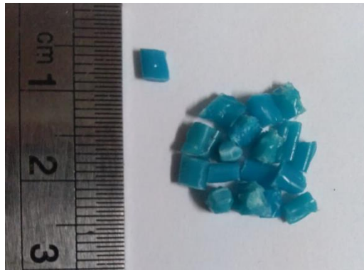
Figure 8. Recycled plastic pellet obtained from 3-ply disposable face mask wastes
