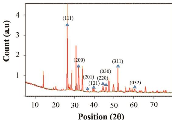
Figure 5. XRD pattern of  $\alpha$ -PbO nanocrystal
