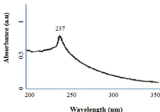
**Figure 2.** UV-Vis spectrum of  $\alpha$ -PbO nanocrystal
