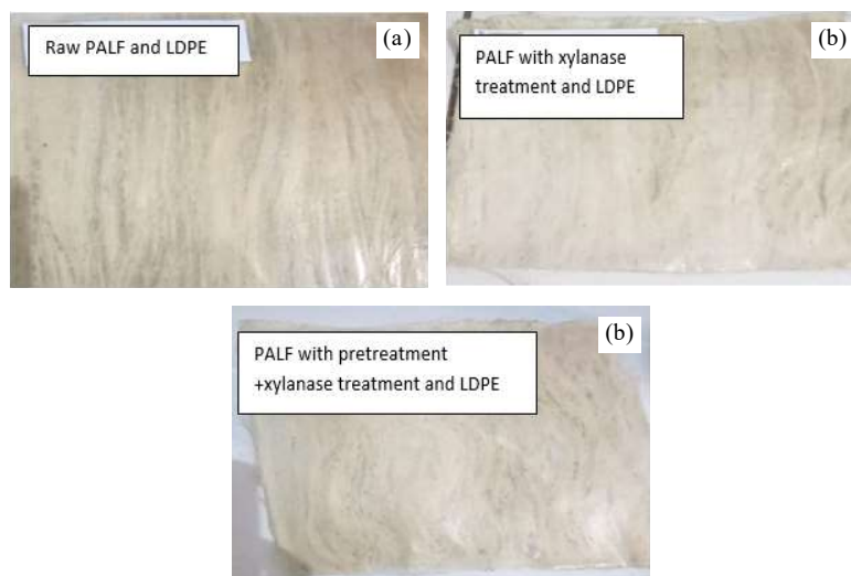
Figure 2. PALF composites (a) raw PALF+LDPE (b) PALF with xylanase treatment+ LDPE; (c) PALF with pretreatment + xylanase treatment + LDPE.
