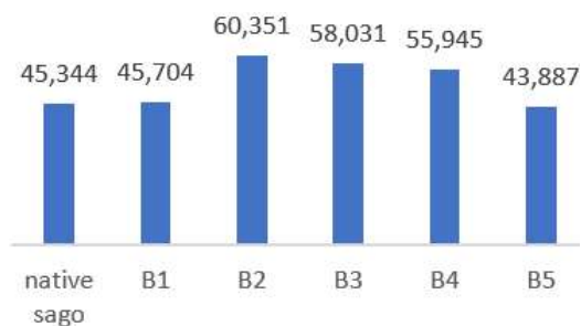
Figure 2. Contact angle analysis of edible film from native and modified sago.
