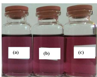
Figure 2. Colloid of Gold Nanoparticles with Various Concentration of HAuCl 4 (a). 3x10 -4 M, (b). 5x10 -4 M, and (c). 7x10 -4 M
