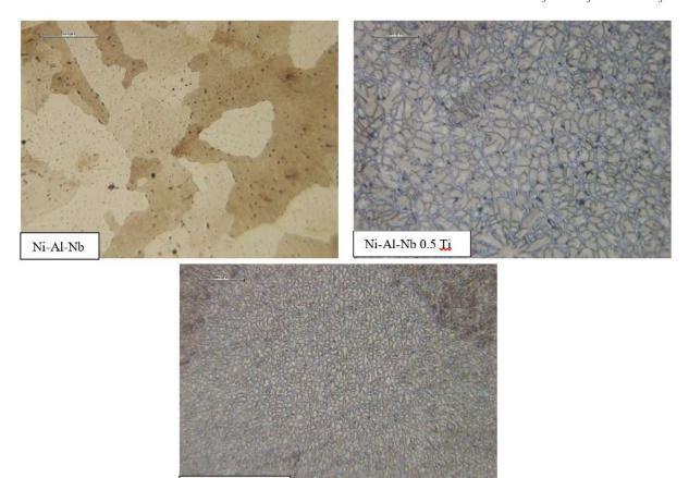
Figure 1. Microstructure 3 different alloys Ni-Al-Nb, Ni-Al-Nb-0.5% Ti, Ni-Al-Nb-1% Ti after solution treatment at 1200 °C for 2 hours 100x
