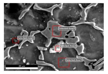
Figure 4. SEM alloys Ni-Al-Nb-Ti 1% after Aging 750 °C SEM
