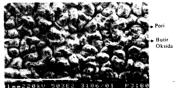
Gambar 11. Hasil SEM sampel A DBANI perbesaran 500 X
