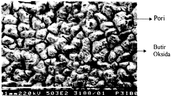
Gambar 12. Hasil SEM sampel A perbesaran 500X
