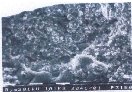
Gambar 1. SrM 40% + PE 60% + 10 mL silane (SEM perbesaran 1010 X)
