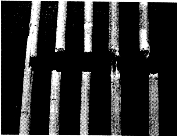
Figure 4. Typical tensile fractures with full breaking
