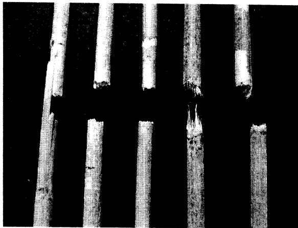
Figure 4. Typical tensile fractures with full breaking
