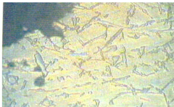
Gambar 6. Struktur mikro flens hasil sandcasting
