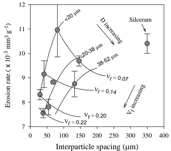
Figure 11. Effect of volume fraction ( $V_f$ ) and particle size (diameter  $D$ ) of TiC reinforcement on the erosion performance of Silceram composites [32]
