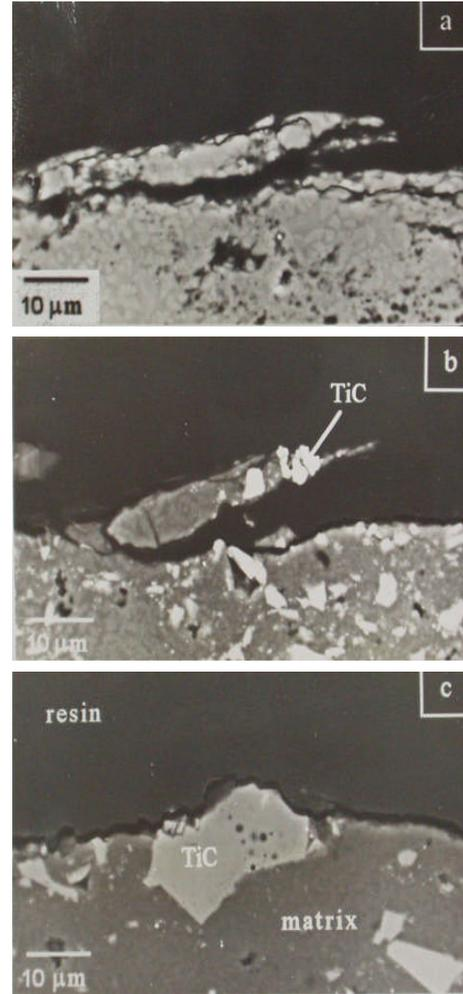
Figure 10. Cross-section of eroded surface of hot pressed Silceram and Silceram reinforced with particulate TiC (a) Monolithic Silceram (b) small (<20  $\mu\text{m}$ ) TiC particles (c) large (20-38  $\mu\text{m}$ ) TiC particles [32]
