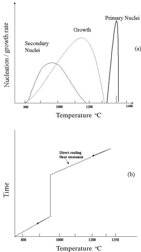
**Figure 4.** Production of glass-based Silceram glass-ceramic by direct cooling and a single-stage heat treatment (a) temperature dependence of the nucleation and growth rates with significant overlap (b) direct cooling/ heat treatment [adapted from 16,17]
