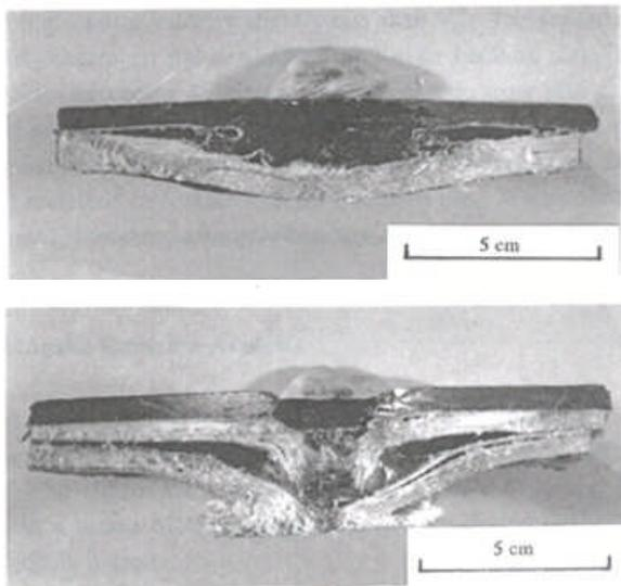
**Figure 6.** Cross-section of a ballistically impacted Silceram-Kevlar armour system of areal density 22.4kg/m<sup>2</sup> after impact with 7.62mm ball round at (a) 619 m/s and (b) 830m/s (the Silceram front face is on the top in these photographs) [22]
