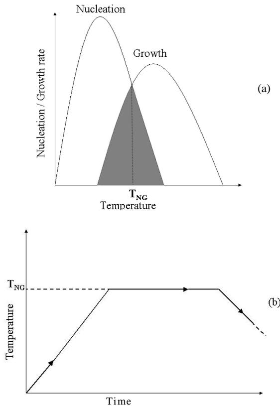
**Figure 2.** Crystallization of glass to form a glass-ceramic by a single-stage heat treatment (a) temperature dependence of the nucleation and growth rates with significant overlap (b) single-stage heat treatment.
