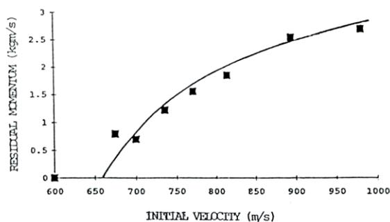
**Figure 7.** Graph of residual momentum plotted against the initial impact velocity of the projectile for Silceram-Kevlar armour system of areal density 22.4kg/m<sup>2</sup> [21]
