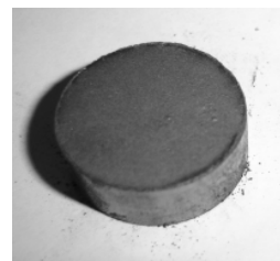
Figure 7. Powder Metalurgi Bipolar Grafit capsule
