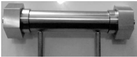
Figure 12. SS compartment of steam reforming methane
