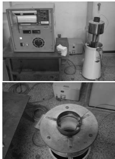
Figure 2. Small scale cylindrical furnace apparatus.
