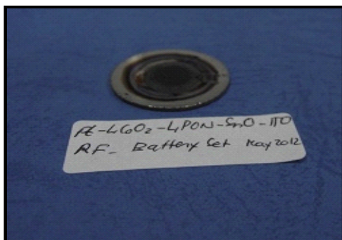
Figure 11. A set of a thin film rechargeable battery prepared by RF Sputtering method
