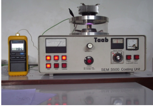
Figure 2. DC Sputtering device in operation at 800 Volt, 30 mA using Argon as sputtering gas with colored glowing plasma showing in the picture
