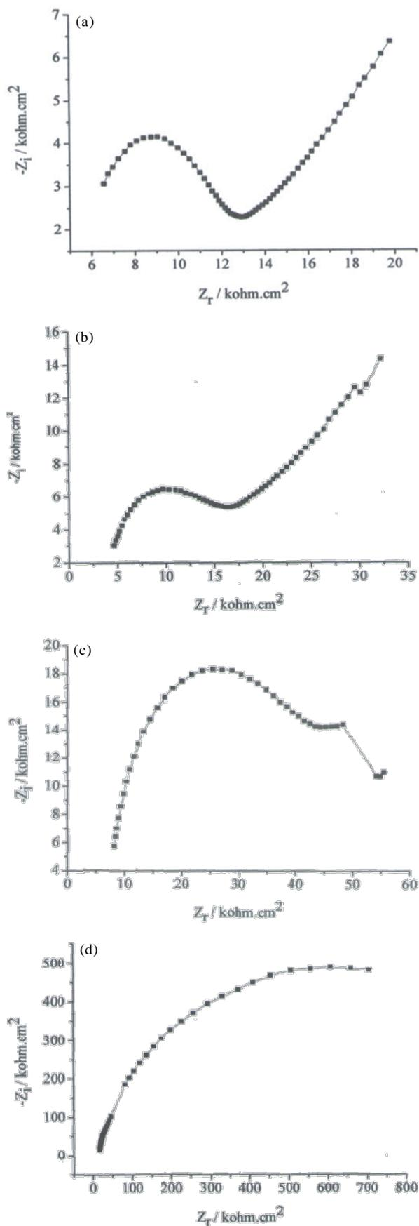
Figure 9. Nyquist plot of (a). M1 membrane, (b). M2 membrane, (c). M3 membrane, and (d). M4 membrane.
