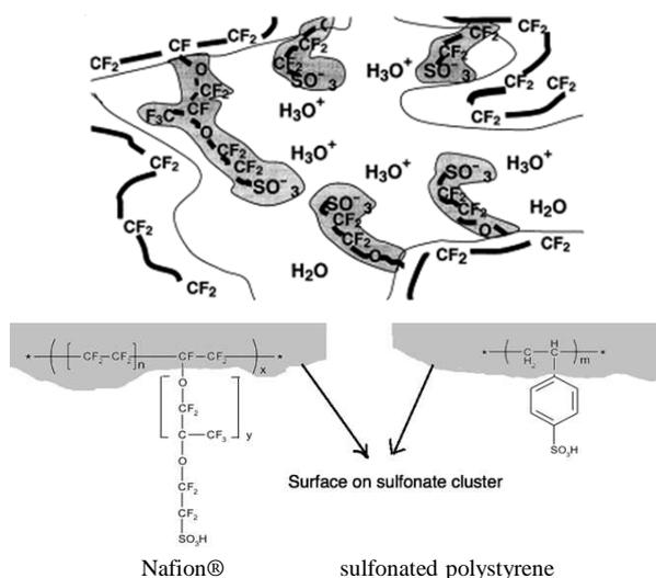
**Figure 1.** Illustration of sulfonate group in sulfonate cluster in Nafion® [2] (a) and the pictorial illustration of comparison between Nafion® and sulfonated polystyrene
