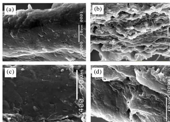
**Figure 5.** Scanning Electron Microscope (SEM) images of cross section of membranes prepared using approach applied in this paper: (a) M1 membrane, (b) M2 membrane, (c) M3 membrane and (d) M4 membrane.
