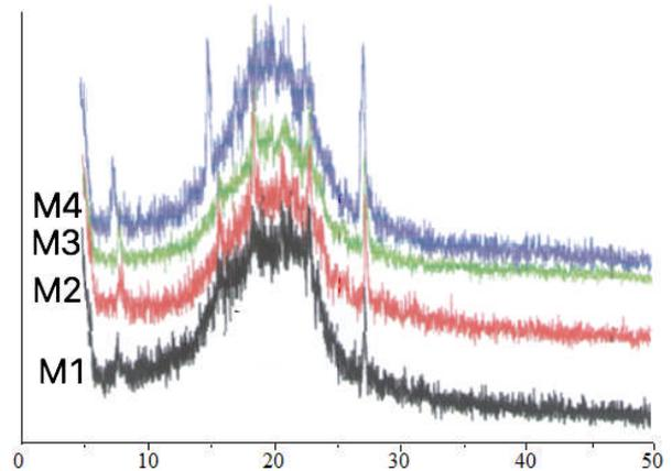
Figure 7. X-RD Diffractogram of membranes prepared using approach applied in this paper M1 membrane, M2 membrane 2, M3 membrane, and M4 membrane.
