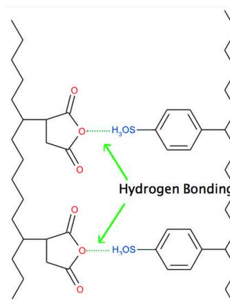
**Figure 2.** Pictorial description of supramolecular structure building by hydrogen bonding between sulfonate group in sulfonated polystyrene and anhydride group in polyethylene-graft-maleic anhydride (PE-g-MAH) along their polymer backbone.
