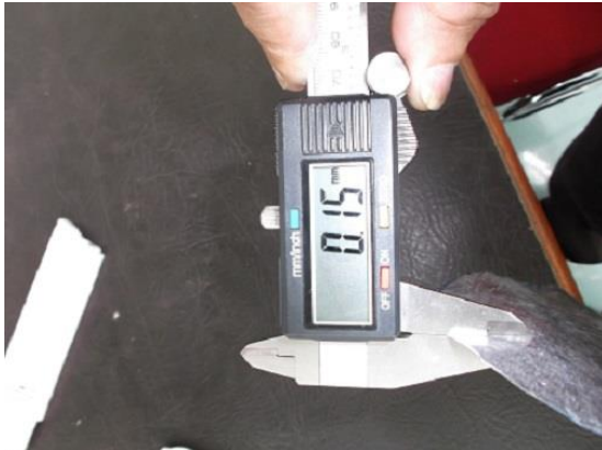
Gambar 1. Tebal filter sreen Pb 0,15 mm.
