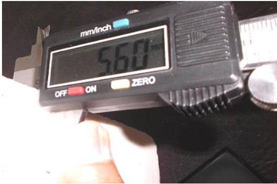
Gambar 4. Tebal Terumbu Karang 5,60 mm. Gambar 5. Window tanpa filter screen Pb.
