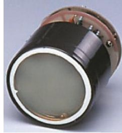
Gambar 7. PSPMT Hamamatsu tipe R2486 [4]
