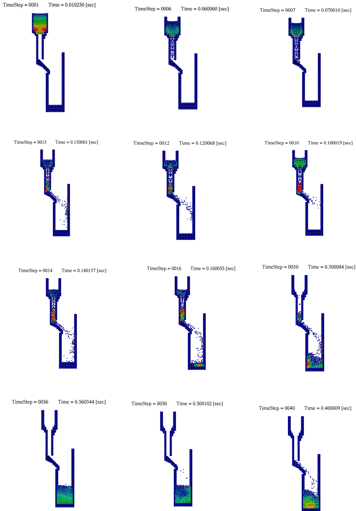
Figure 8. Pressure Profile of Candle Wax relocation process.
