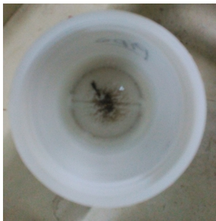
Figure 4. The Sediment Samples from Heat Exchanger Tube.
