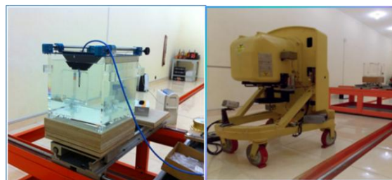
Figure 4. water phantom for calibration (left) and Co-60 source for calibration of therapy level.
