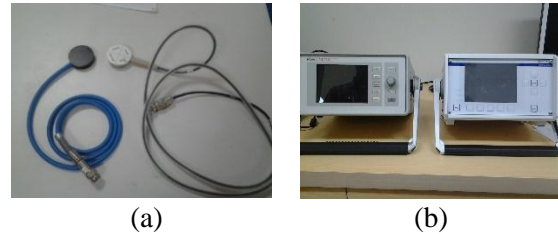
Figure 2. a) PTW Roos and IBA PPC40 ionization chamber b) PTW Unidos Webline and IBA Dose 1 Electrometers
