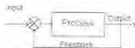
Gambar 2. Proses Kerja Sistem Untaian Tertutup ( Closed Loop )
