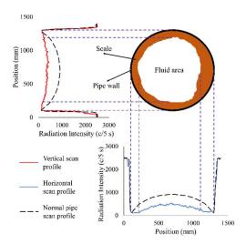
Figure 5. Scale profile prediction at point Q.
