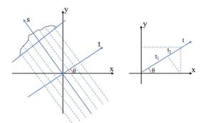
Figure 1. Parallel beam geometry [6].
