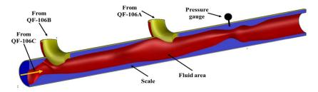
Figure 6. Three-dimensional scale profile prediction along BA-106 pipeline.
