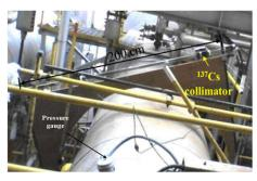
**Figure 4.** Gamma tomography scanning system set up in the field.
