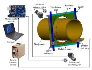
Figure 2. Gamma tomography scanning and data acquisition system schematic [22].
