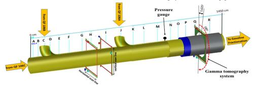
Figure 3. Gamma pipe scanning and tomography positions.
